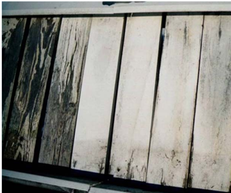
Figure 2: Performance of acetylated coated panels after 13 years of exposure. The 4 panels on the right hand are acetylated and the others are unmodified controls. Prior to testing the panels were coated with alkyd primer followed by acrylic top coating
