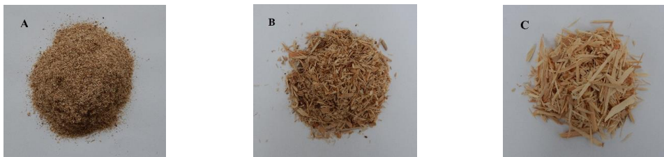
Figure 1: Particle used in particleboard. A – surface particle, B – core particle (normally used in PB), C – sub-dimensional particle from OSB production used in core layer.
