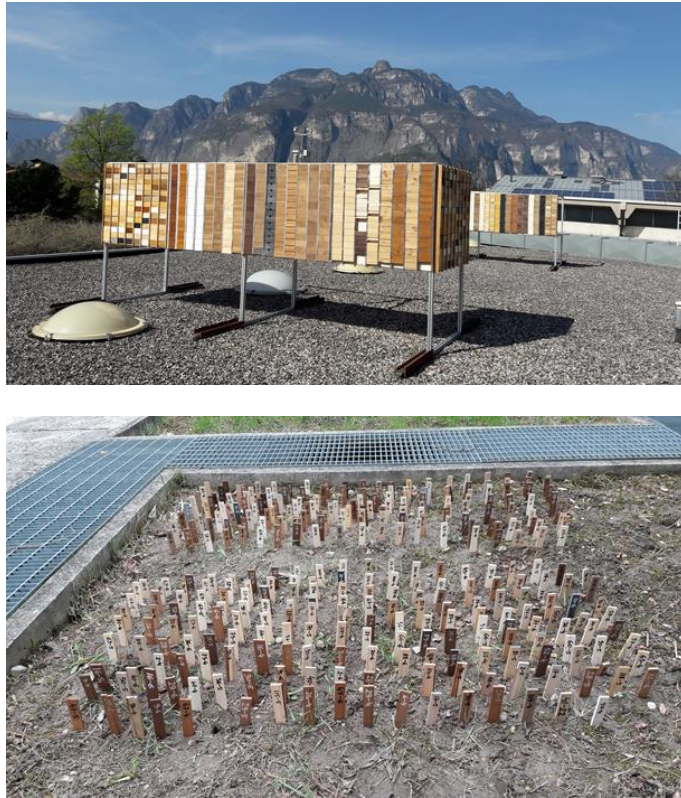
Figure 1: Facades materials exposed to natural weathering (up) and during degradation in soil – simulation of landfilling (down)
