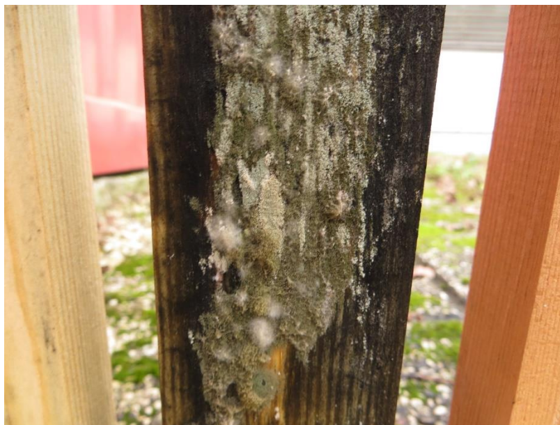
Figure 1: Growth of blue stain and mould fungi on Scots pine sapwood samples exposed in Ljubljana.
