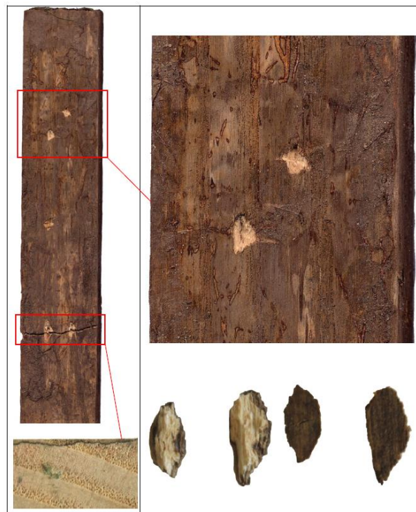
Fig. 3: European ash. Failure after 0.5 years exposure. Visual inspection showed typical signs of soft rot: shell-shaped splinter, attack on the outer wood shell, clean fracture.
