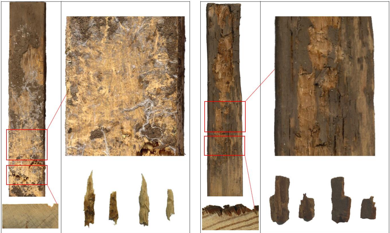
Fig. 2: Left: Beech. Failure after 0.5 years exposure. Visual inspection showed typical signs of white rot: whitish discoloration, long-fibred splinter, fibred fracture. Right: Southern yellow pine. Failure after 0.5 years exposure. Visual inspection showed typical signs of brown rot: brownish discoloration, brittle/cubical splinter, cross-checking texture
