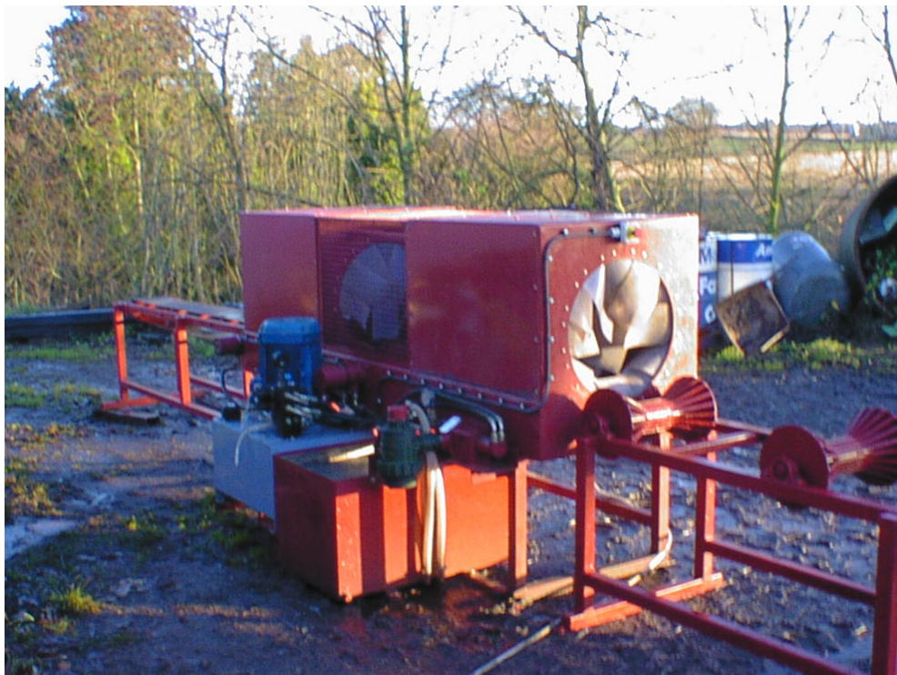
Fig.2: Pilot pre-treatment plant; poles/logs are drawn through the plant while being steam sterilised and inoculated.
