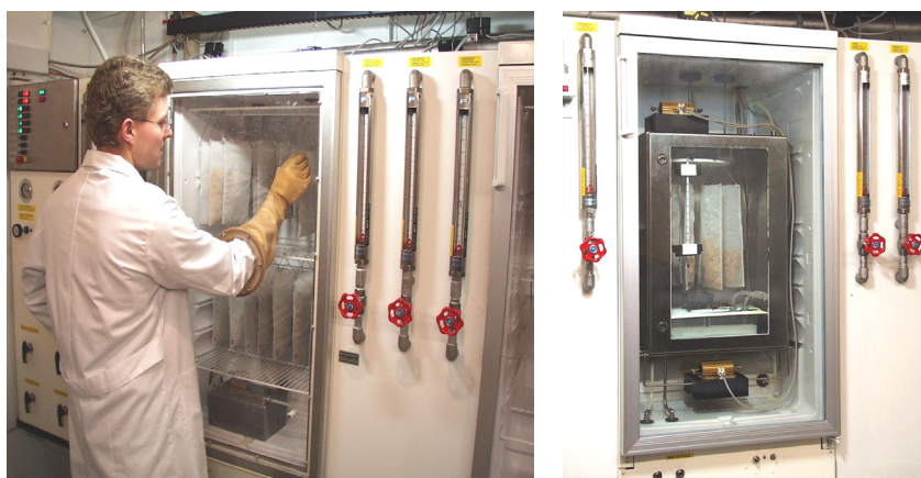
Figure 2: New climate chambers for improved sorption studies.
