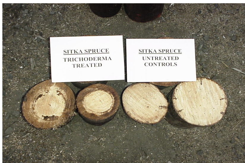
Fig. 3: Sectioned logs of Norway spruce after fungal pre-treatment with T. aureoviride , incubation at ambient temperature, drying and subsequent and creosote treatment.
