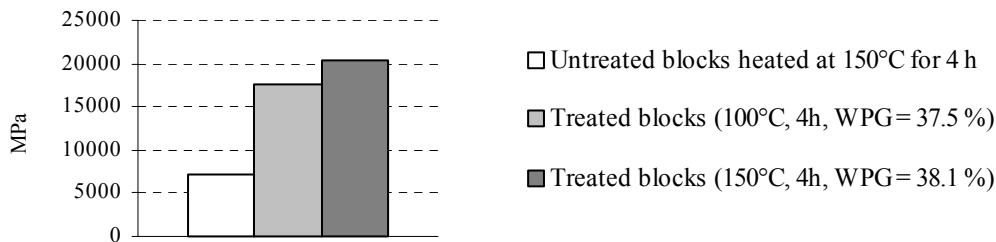
Figure 3: Modulus of elasticity of untreated and treated with aqueous solution of PG/MA adduct (30 %) in the presence of MEKP (2 %) and cobalt naphthenate (2 %) pine blocks
