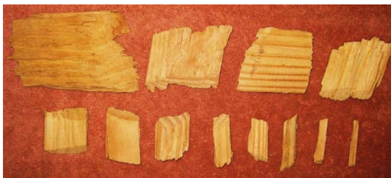
Figure 1: Southern pine chips of various sizes used for acetylation.
