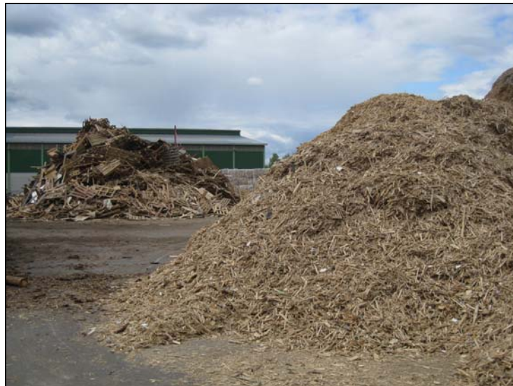
Figure 2: Recovered solid wood is often chipped for burning in the Nordic countries. Its moisture content is low which makes it very desirable material for heat and power production. The same material could easily be utilised in selected wood products, as well. Photo: Henrik Heräjürvi.
