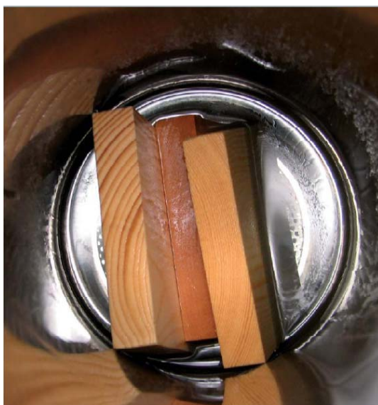
Figure 3: Wood samples after scCO 2 impregnation
