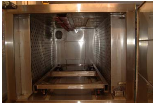
Figure 2: Typical small scale heat treatment oven used in Wales
