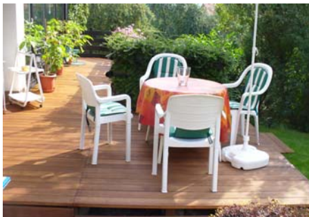
Figure 3: Decking elements and picnic benches made from DMDHEU treated Beech wood
