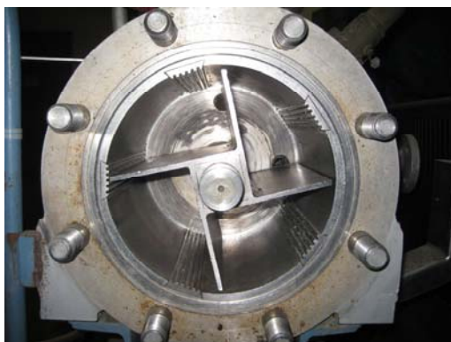
Figure 3: Asplund Defibrator with 0.7 mm gap
