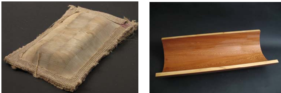
Figure 5: Moulded end grain board (a) and uniaxial densified half pipe (b)
