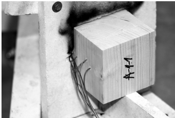
Figure 1: The wood specimen with thermocouples fitting in sample holder with removed thermo-isolation
