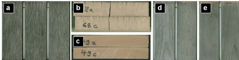
Figure 2: Specimens after two years of weathering. a) Surfaces of native beech. b) Cut references. c) Cut specimens of wax impregnated wood. d) Surface of impregnated beech with wax 1 and e) wax 2
