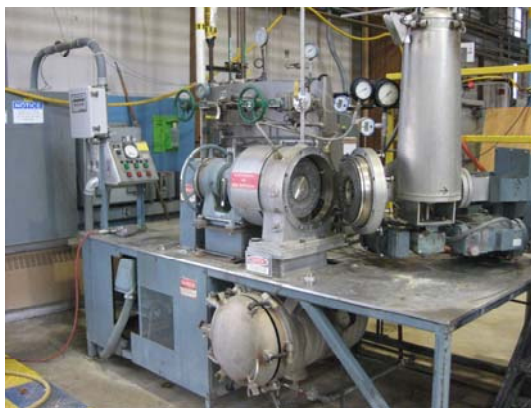
Figure 4: Sprout-Bauer double disc, pressurized refiner
