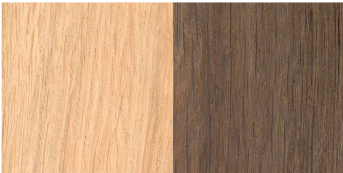
Figure 1: Colour change of oak wood due to ammoniation (left: reference, right: ammoniated)
