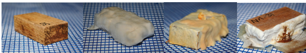
Figure 2: Test fungi (Left to right): Coniophora puteana, Oligoporus placenta, Gloeophyllum trabeum, Trametes versicolor
