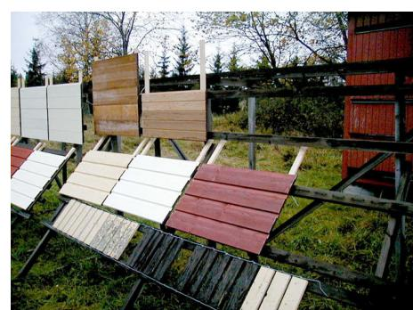
**Figure 4: Natural field weathering of FRT wood panels exposed both vertically and at 45° slope**
