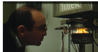
**Figure 2 : Cone calorimeter, ISO 5660, sample size 100 x 100 mm**
