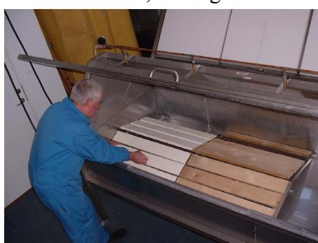
**Figure 3: Accelerated ageing of FRT wood panels according to NT FIRE 053**
