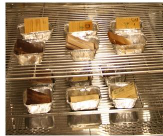
**Figure 1: Hygroscopicity tests according to NT Build 504**
