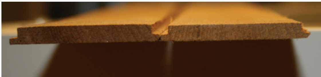
Figure 2: Two profiled ribs used for adhesion tests of the sealant
