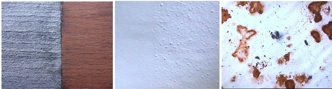
Figure 2: Natural weathering (left); compatibility with mortar (middle) and with metal (right)
