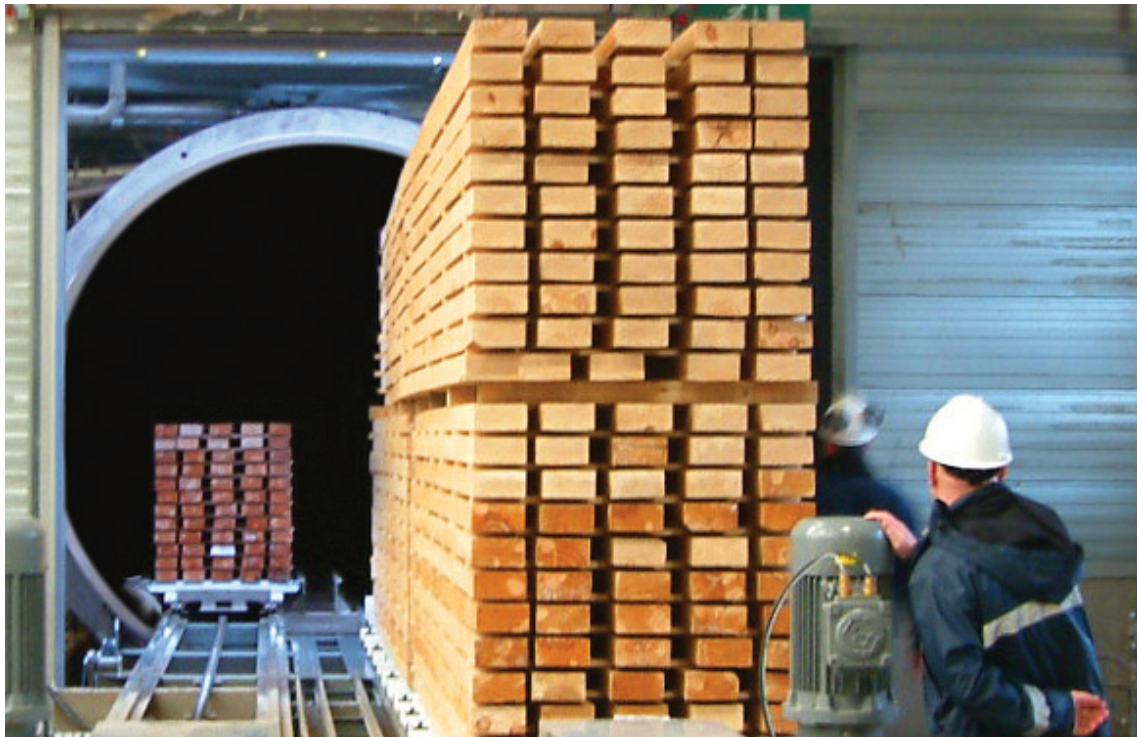
Figure 1: Commercial acetylation plant of Titan Wood
