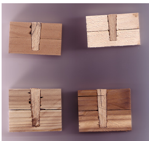
Figure 3 : Fixation of dowels within Sitka spruce samples. Anticlockwise from top right: control, heat treated, acetylated, furfurylated
