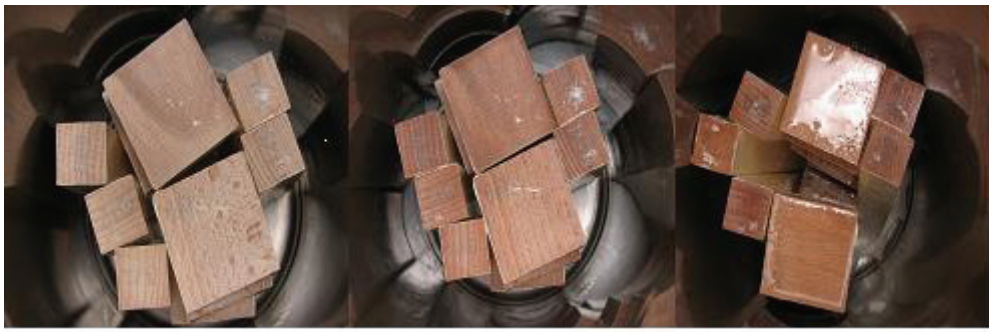
Figure 4: Beech specimen before and after scCO 2 impregnation
