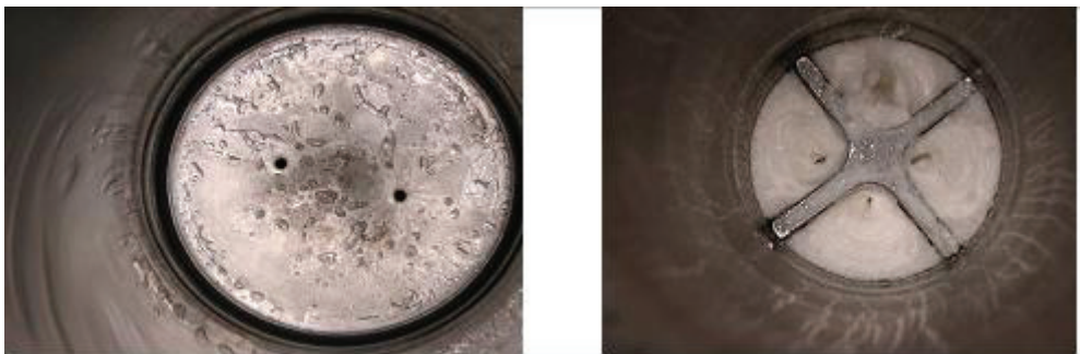
Figure 5: Precipitated silica sol particles in Vessel V1
