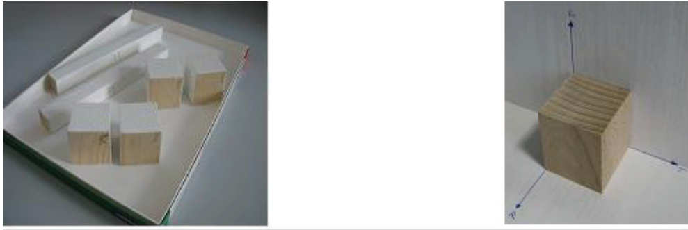
Figure 3: Specimen for determining intrusion depth
