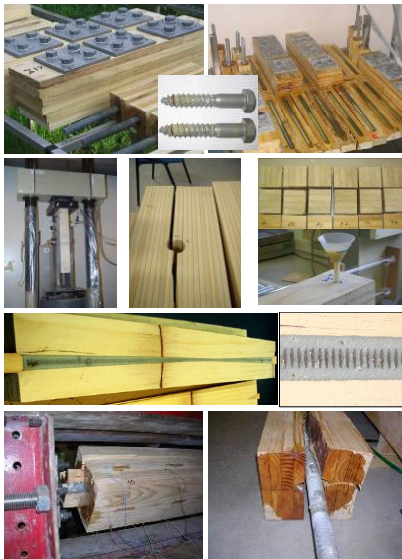
Figure2: Some of the test samples used in the extensive research and test program; corrosion test, mechanical testing of the wood, lamination and in-glued rod connections, resin injection trials.
