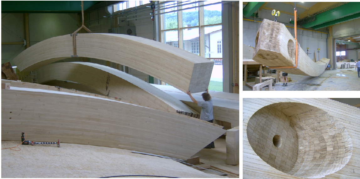
Figure 4: Elements with cross cut of 1,4 by 1,1 meter, double banded. Profiled for specific rotating connection between the horizontal carrier and the vertical pressure bow.
