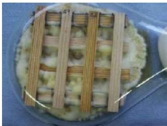
Figure 1: Kollé flask with *C. puteana* and ENV 807 samples (four oil-treated, four controls)
