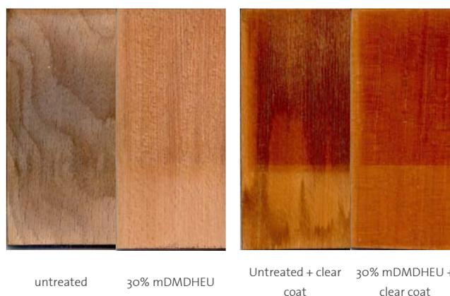
Figure 12: Surface quality after 3 cycles of accelerated weathering in the QUV-tester
