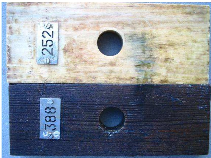
Figure 3: Oil Heat Treated (sound) and Acety+MMF, 21+8 (sound) after 5 years.
