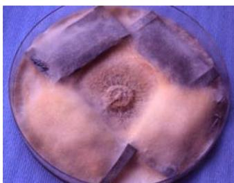
Figure 2: Wood particles in stainless steel bags in polystyrene Petri dishes (lid removed) with *C. puteana*. Modified particles in upper bags – controls in lower bags
