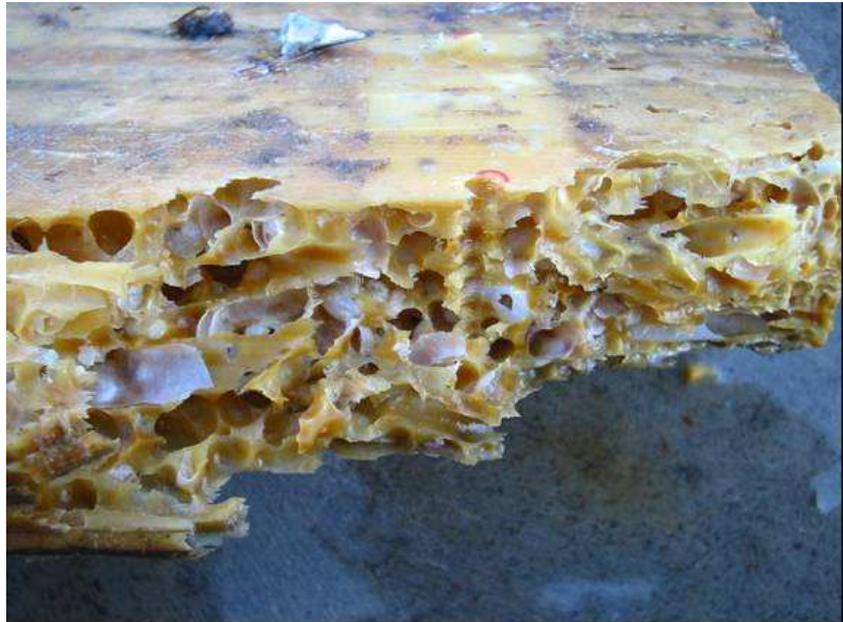
Figure 1: Control sample (failed due to Teredo attack) that broke when being removed from the rig.
