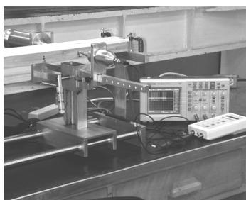
Figure 1: Acousto-ultrasonic Apparatus
