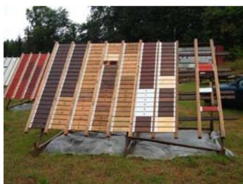
Figure 2: Field exposure of coated panels according to EN 927-3 in the Bogesund field
