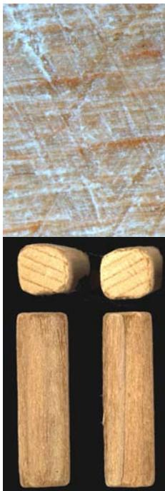
Figure 7: Abrased specimens: left: surface of a heat treated beech specimen after 1000 rounds in the Taber abraser (x10); right: heat treated silver fir specimens after 72 h abrasion in the shaker
