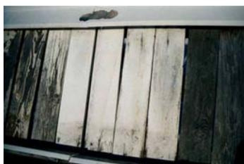
Figure 1: 13 year old field test of acetylated (the 4 panels in the middle) and unmodified wood panels (the 2 panels to the right) coated with alkyd primer followed by acrylic top coating.
