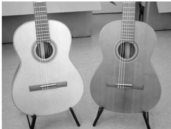
Figure 9: Guitar made of thermally modified spruce (right) und unmodified spruce (left)
