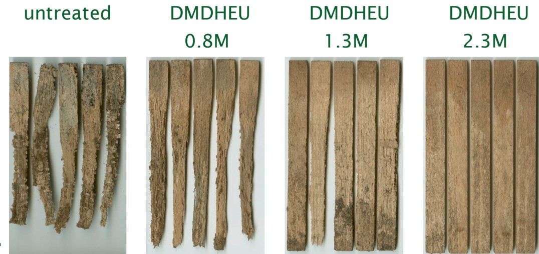
Durability test in ground contact following DIN V ENV 807 (152 weeks)
