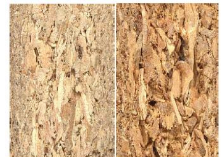
Particle boards glued with PMDI (Bartholme 2005)
