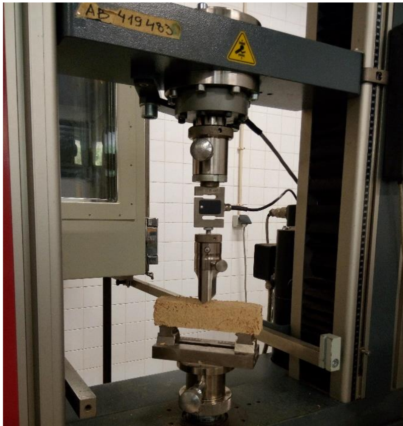
Zwick Rowell Z050 equipment Support distance: 100 mm
