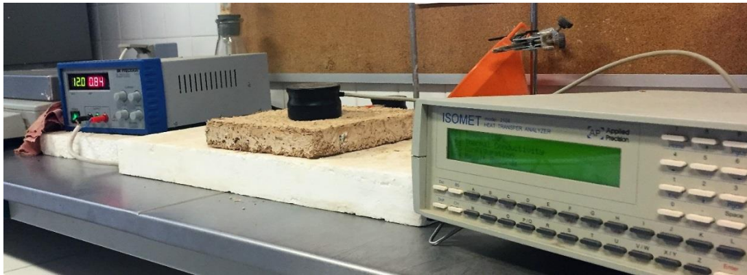
ISOMET 2104 Heat Transfer Analyzer equipment and contact probe
