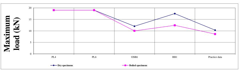
Bonding test of the four formwork composites depending on the alternative surface layers used (Zwick/Roell Z020)
