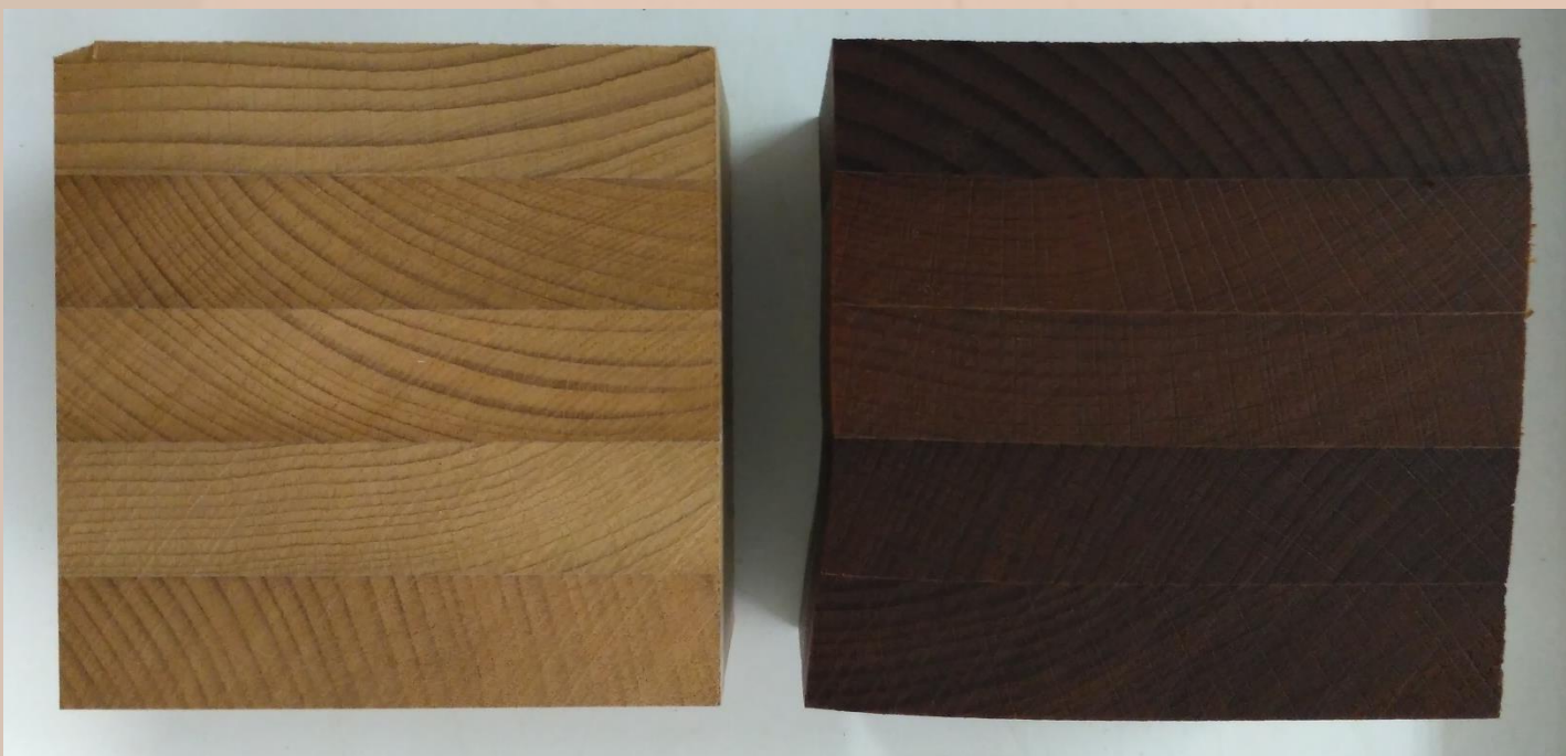
Thermally modified beech wood samples before (left) and after impregnation (right).
