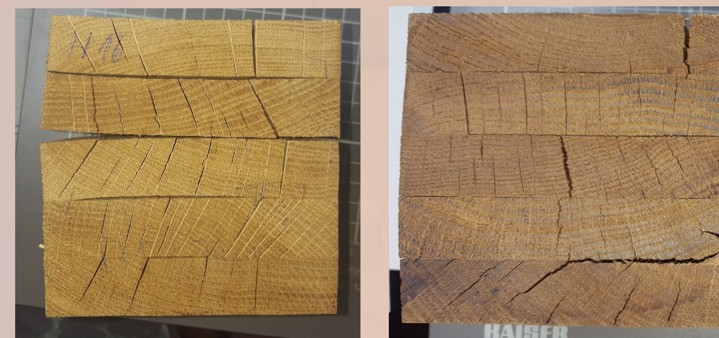
Extreme delamination of unmodified and thermally modified oak wood samples.
