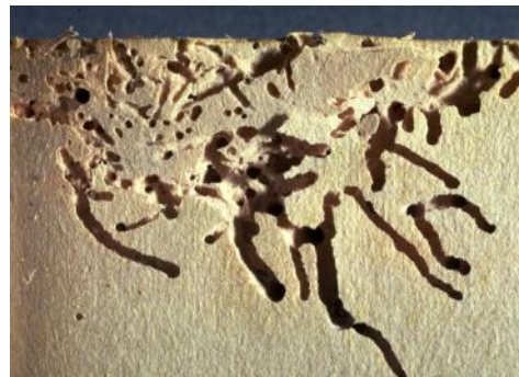
Compressed paper degraded by Anobium punctatum
