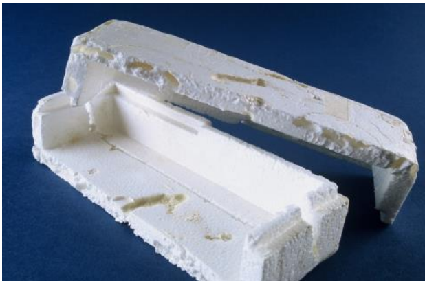
Polystyrene degraded by Hylotrupes bajulus
