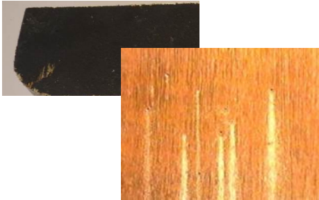
Plywood panels infested by Lyctus sp.
