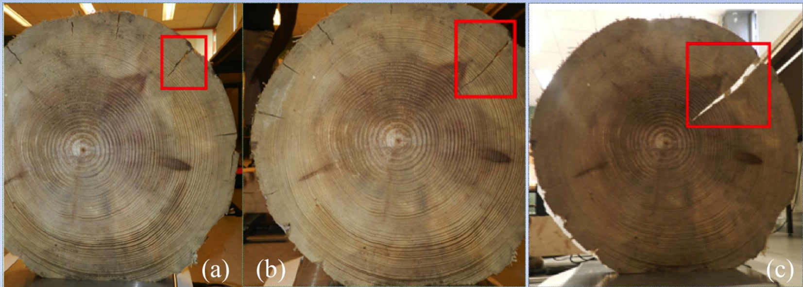
Fig. 1 : Slice cracking induced by natural drying of white fir slice
