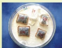
Figure 2: Mycological test of polysaccharide thermal insulations against Serpula lacrymans (S.1.)
