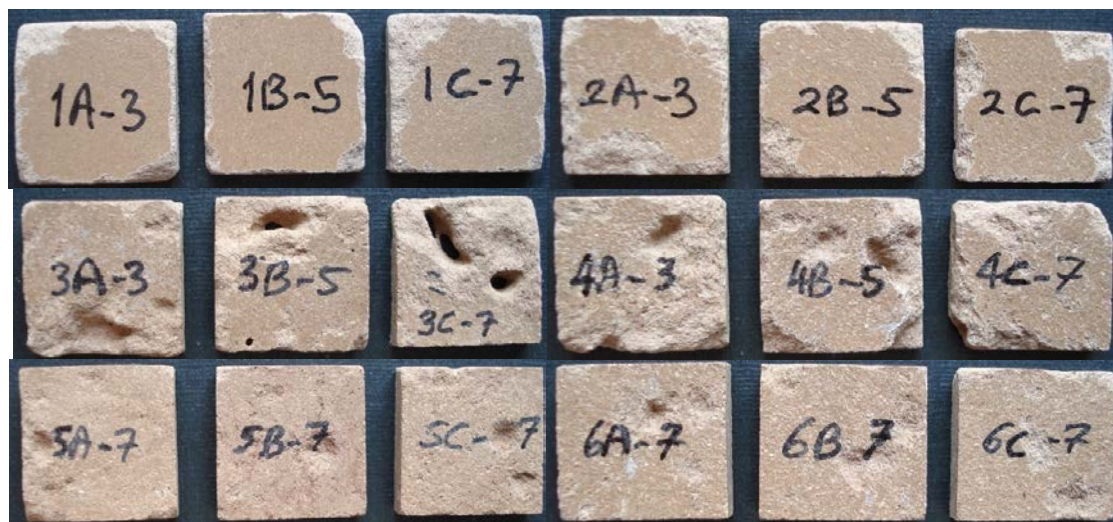
Figure 1: Typical damage modes of laboratory termite activity on representative specimens from all WPC formulations tested.
