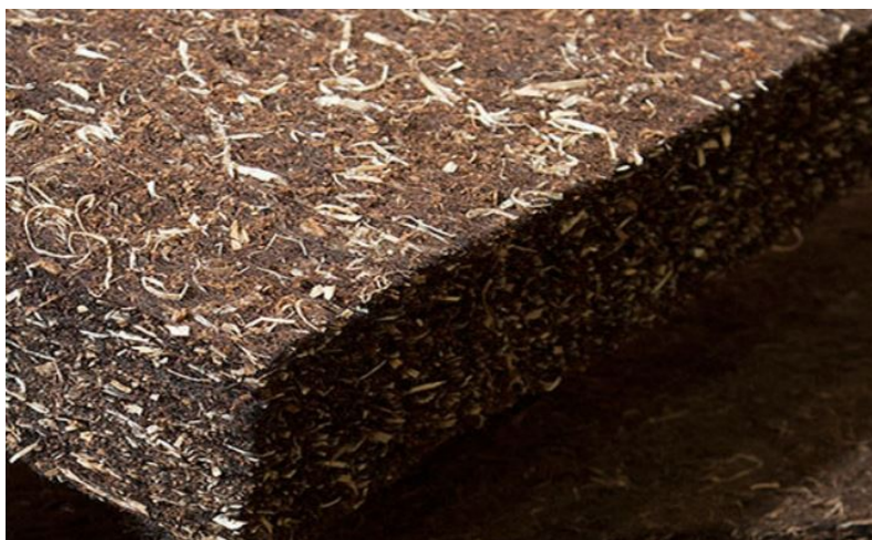
Figure 2. Konto-insulation plate of peat and timber fibre; #50 and 75mm (Konto OY)
