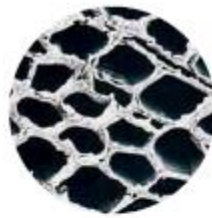
Photograph, taken through an electronic microscope, showing a section of a thin layer of fir wood-wool taken from a standard panel (Padua University, 1995).
