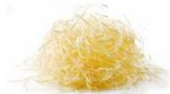
50% of Celenit is made up of long, strong fir fibres.
