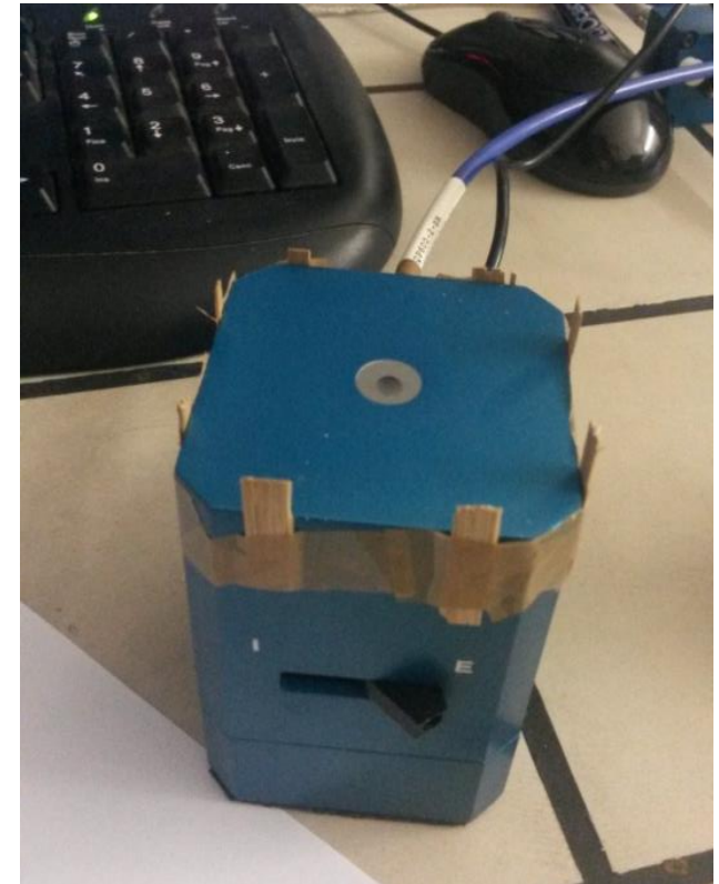
Modified probe for the acquisition of UV-VIS spectra acquisition using integration sphere
