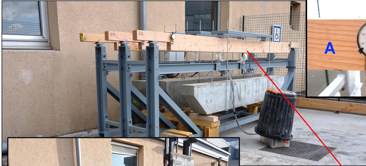
Comparator To measure the crack opening
