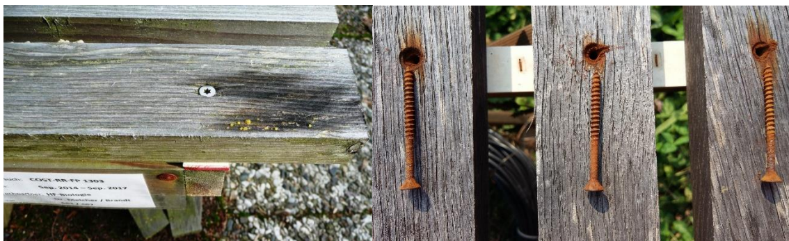
Figure 1: Fruit bodies of Dacrymyces spp. on Norway spruce specimens exposed in Hamburg (left) and corrosion of galvanized screws on English oak specimens exposed in Ljubljana (right) after two years of exposure.
