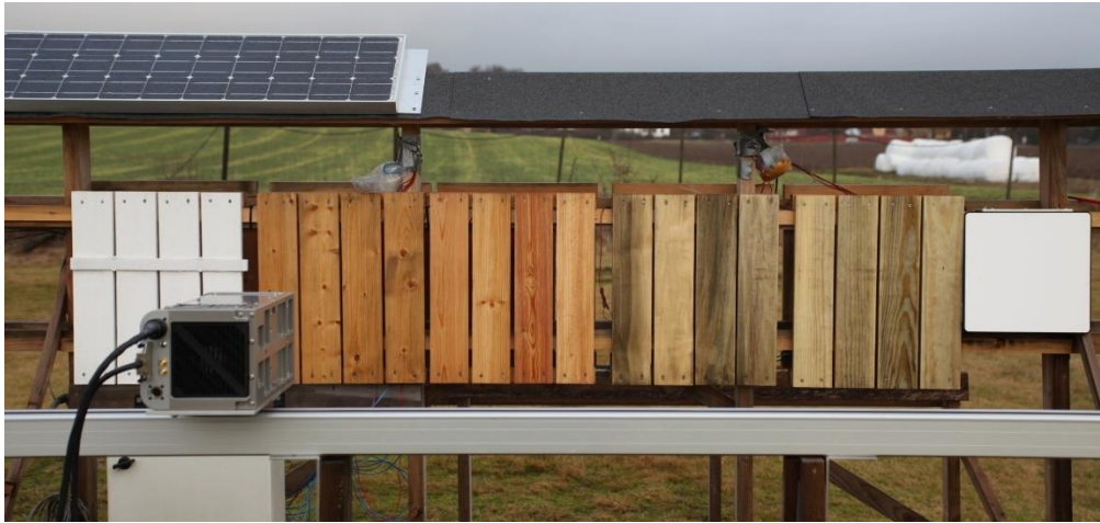
Figure 1: Experimental outdoor setup with five different wood substrates facing south, a white reference Spectralon and hyperspectral camera setup (left to right; coated spruce, spruce, pine, aspen, acetylated spruce).
