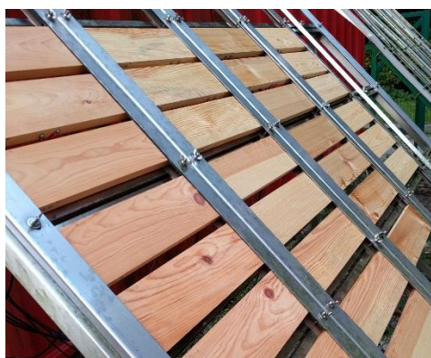
Figure1: Exposure of the samples to natural weathering on the field test site in Ljubljana
