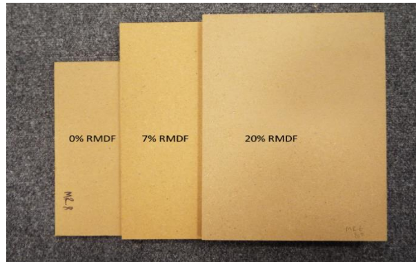
Figure 1: Panels manufactured with different additions of rMDF fibre
