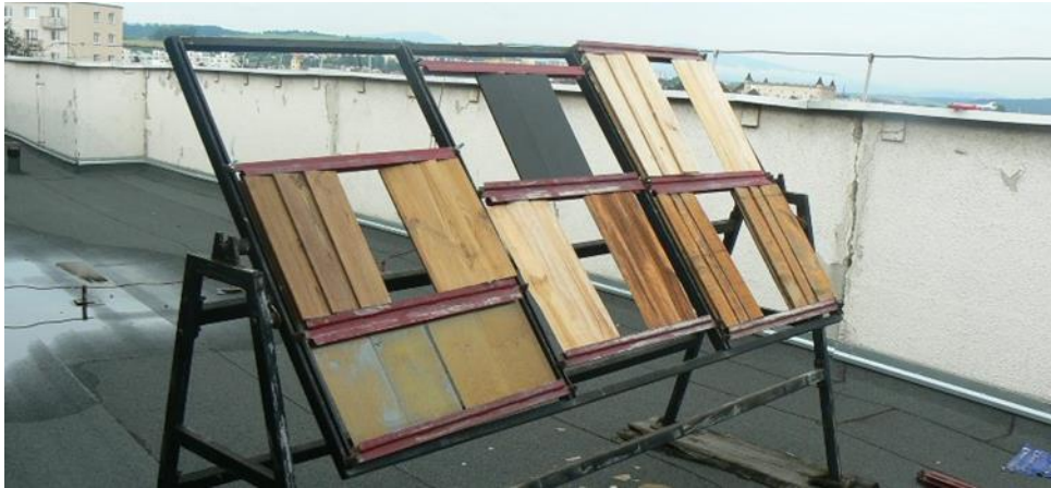
Figure 1: Natural ageing of wooden shingles in the exterior exposure under a 45° slope orientated to the South at Technical University in Zvolen (from July to April)
