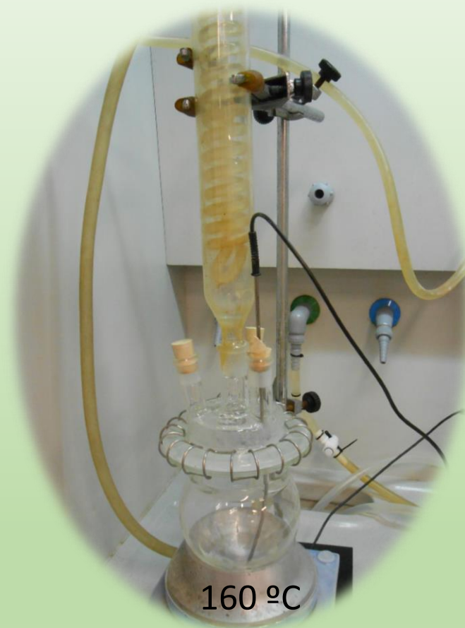
Figure 1 – Reaction conditions of liquefaction under reflux
