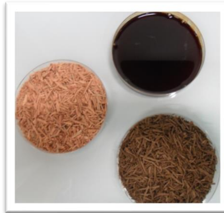
Figure 4- The wood, black liquor and pulp unbleached pulp by Organosolv process.
