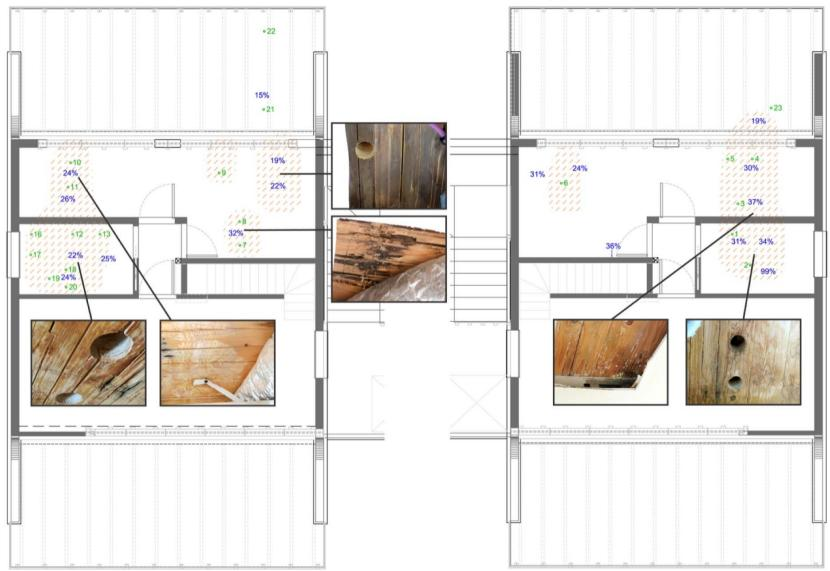
There is a correspondence between the high moisture content and the developing of fungal attack as evidenced by the photos.
