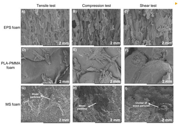
For PLA-PMMA, the fracture occurs inbetween precursors
