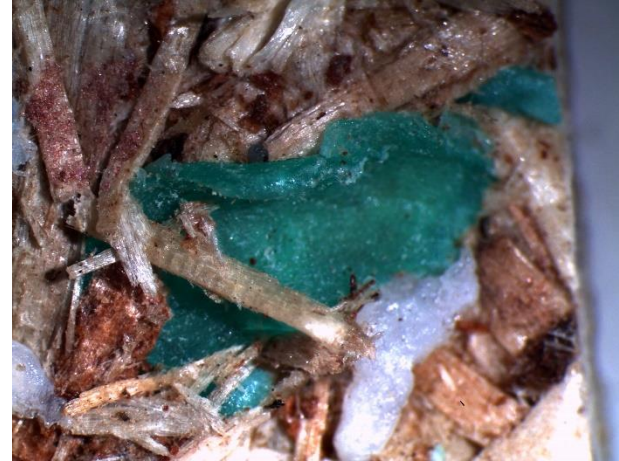
Middle layer of particleboard after the tensile strength perpendicular to plane.
