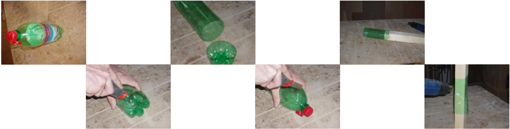
Scheme of manufacturing of surface treatment from PET bottles
