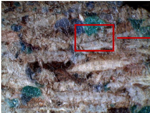
On side particleboard containing 30 % PET.
