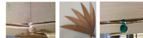
Figure 2. LLBC reinforcement of pine wood, flat shape (on the left) and D-shape (on the right) [Burawska et al. 2015]
