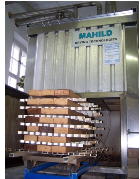
experimental thermo kiln of IHD
