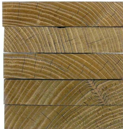
spruce TMT, hardly compression wood
