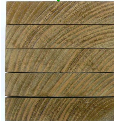
spruce TMT, high amount of compression wood
