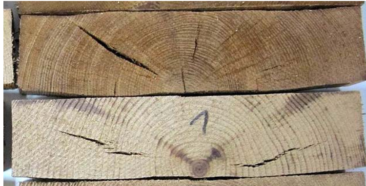
internal cracks, pine TMT; photo: anonym
