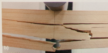
Failure modes observed in (a) group A, (b) group B, (c) group C, and (d) group D
