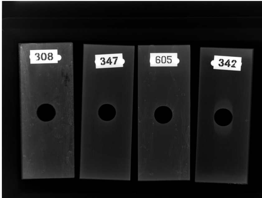
Figure 2: X-rays of boards of treated and untreated wood after submersion in Olhão Harbour, Portugal for six months. Shipworm attack is visible in panel 308(pine control)
