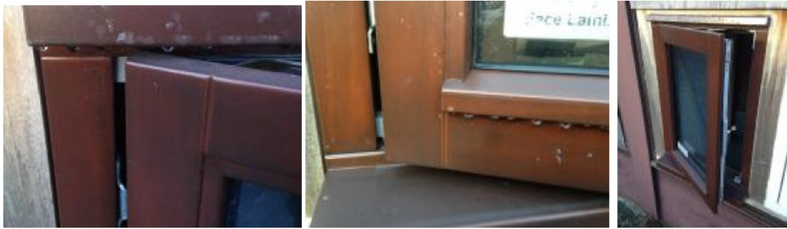
Figure 4: Accoya face-laminated windows, 30 months old on test at the controlled interior climate window exposure site, BRE, UK
