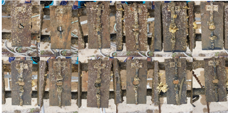
Figure 1: Boards of treated and untreated wood after submersion in Olhão harbour, Portugal for six months
