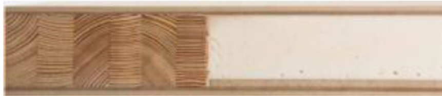
Figure 7: Typical build-up of an engineered door with Tricoya only on the two faces
