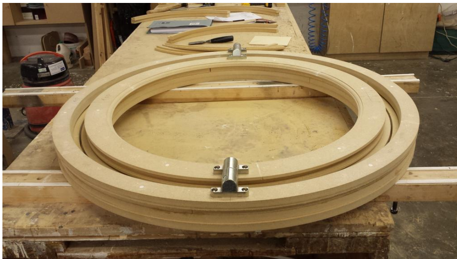
Figure 9: Tricoya complex circular joinery
