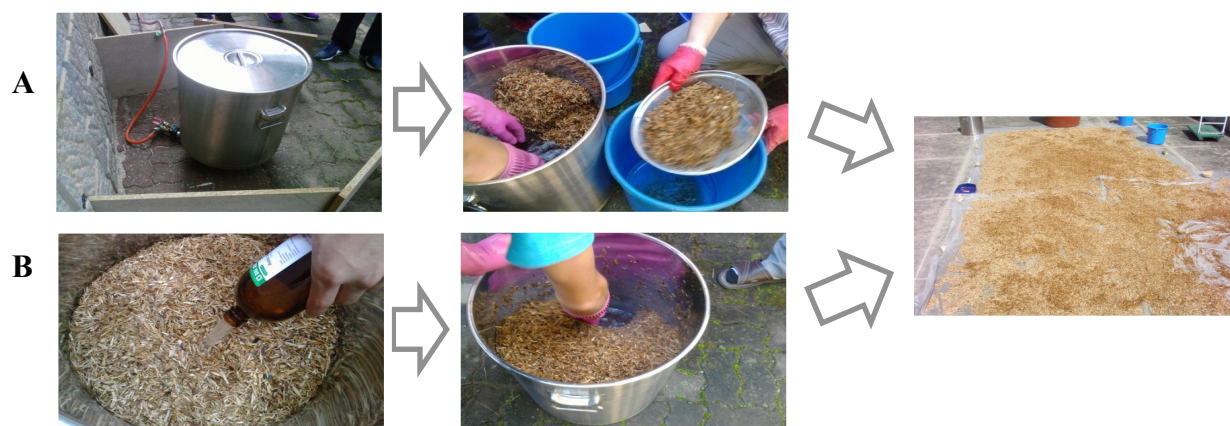
Figure 1: Acetylation of wood particles. A: heating at 100 °C for 1 h, B: room temperature (25 °C) for 48 h
