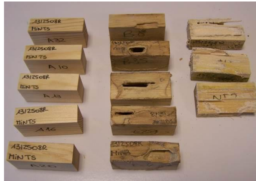
Figure 2: Scots pine samples treated with two solutions with high silica content after being exposed to termites (on the left: HM1; in the middle: HM2; on the right: untreated specimens)
