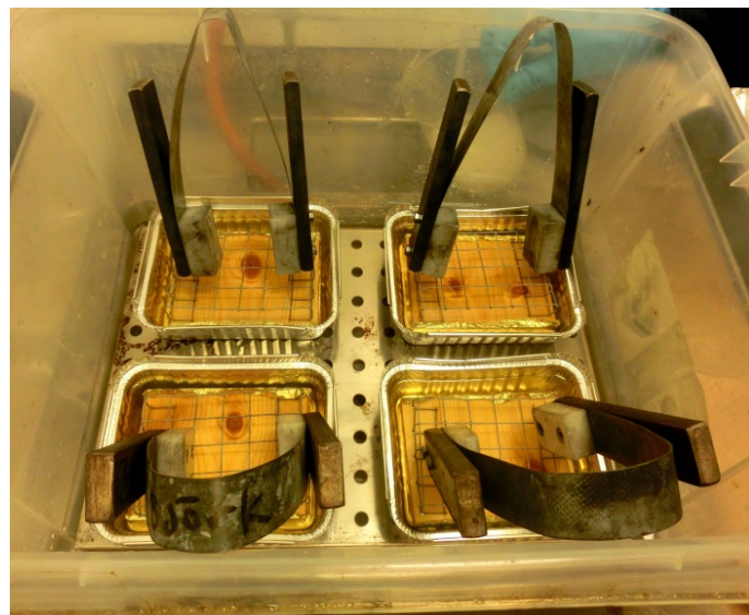
Figure 1: Samples submerged in cold liquid solutions and pressed by loads
