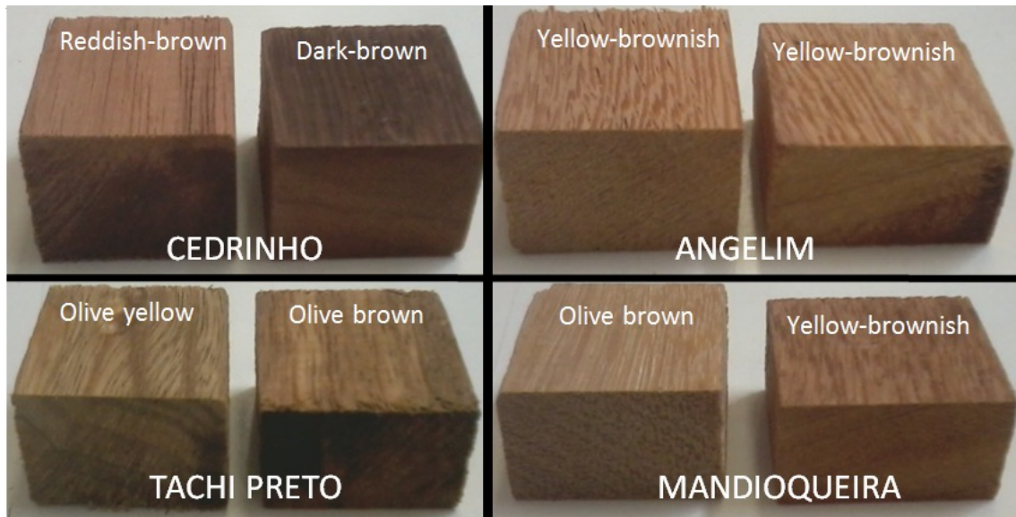
Figure 1: Color of the samples before and after treatment defined according color table from Camargos and Gonzalez (2001)
