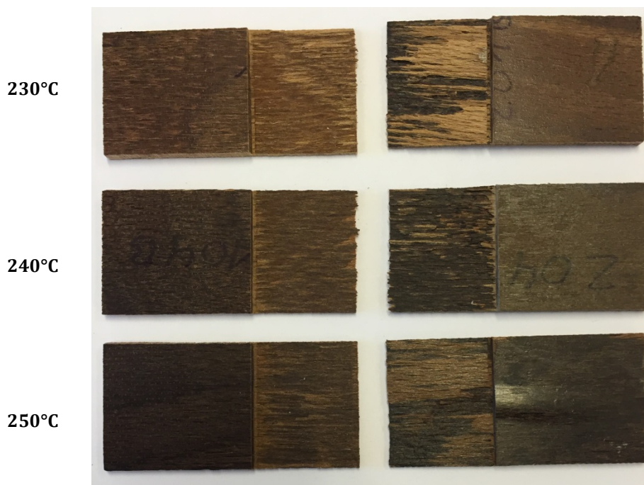
Figure 1: Samples of boards pressed at 230, 240 and 250°C after shear testing. Boards from veneers treated (left) without and (right) with hydrogen peroxide
