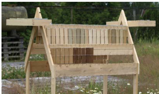
Figure 1: Test set up, vertically exposed samples
