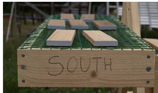
Figure 2: Test set up, horizontally exposed samples
