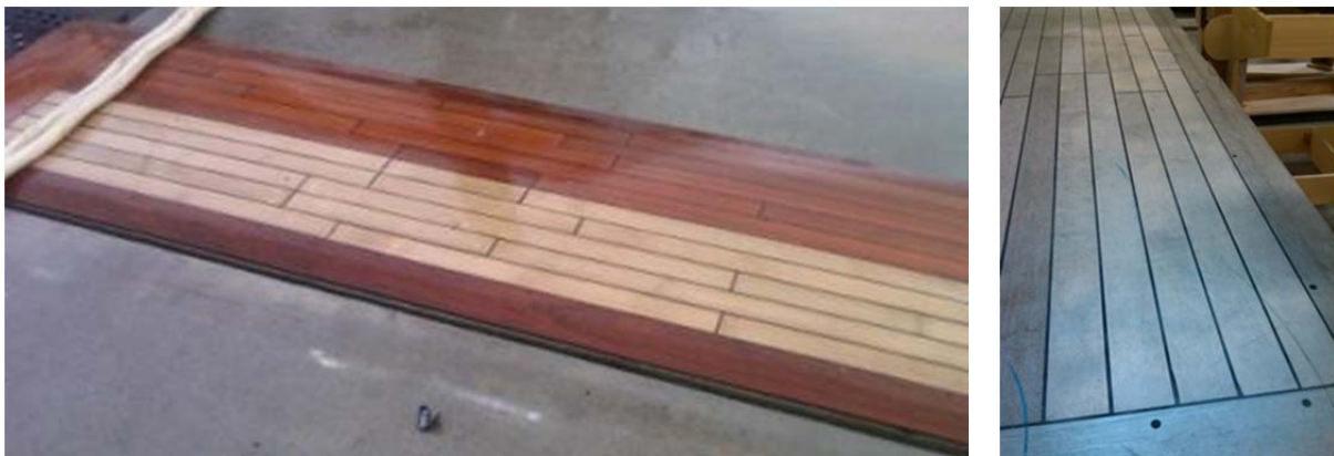
Figure 5: in situ comparison between Burmese Teak and vertical grain acetylated Accoya Alder. Source: Westport shipyard, Port Angeles, WA, USA. Left: At installation; Right: after 10 months weathering
