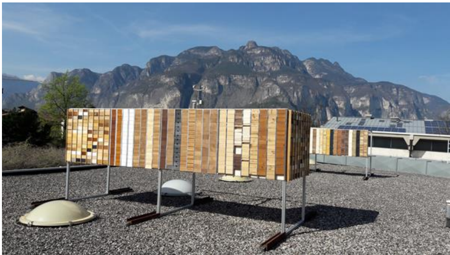
Figure 1: Facades materials exposed to natural weathering
