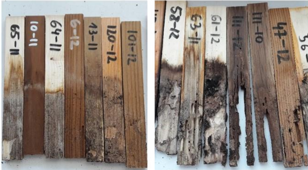
Figure 4: Facades materials after 3 months of degradation with termites in laboratory tests rated according to 5 point scale EN 252 (adapted) (left: grade 2 – moderate attack, right – grade 4 –failure)
