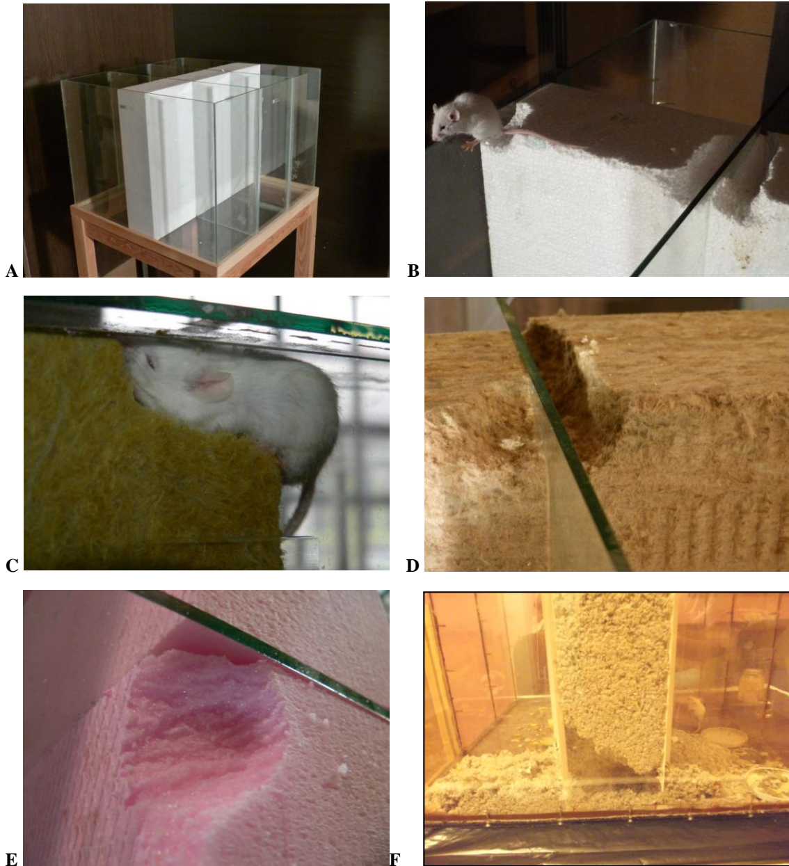
Figure: 1 Examples of the thermal insulations attacks by house mouse males and females: A – glass container divided with two glasses on three 179 mm wide subsections prepared for testing the “EPS 70 F WhiteFacade” insulation; B – attack of expanded polystyrene EPS 70 F WhiteFacade; C – attack of rock-wool Isover TF; D – attack of glass wool Isover Multimax; E – only poor attack of extruded polystyrene Austrotherm XPS TOP; F – strong attack of cellulose insulation Tempelan
