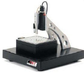
Figure 2 : MicroProf FRT roughness device with the specified scanning parameters
