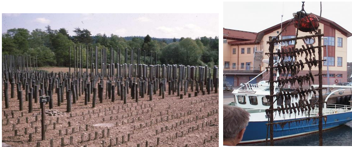
Figure 4. Simlångsdalen “old” test field and rig for marine testing according to EN 275 at Kristineberg on the Swedish west coast.
