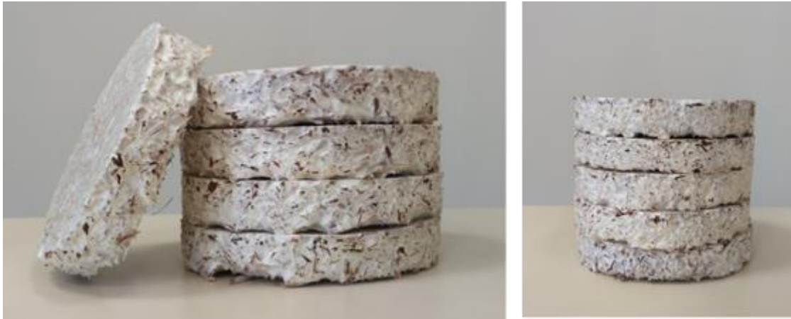
Figure7 : P. ostreatus grown in ø14cm petri dishes with Apple (left) or Vine (right) woodchips.
