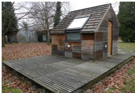
Figure 1: Wooden model house unit in October 2016, after 3 years of exposure.
