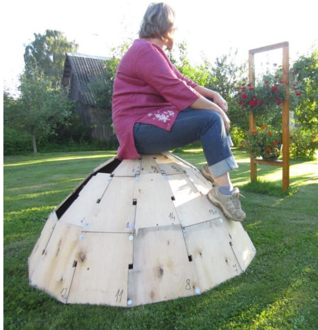
Figure 5: Field test of partly mounted dome-shell. (Photo T.Teppand)
