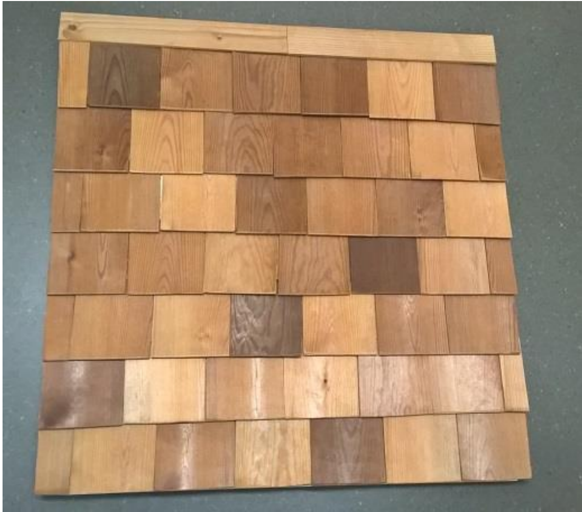
Figure 3: A prototype for shingle shower wall of thermally treated split spruce. Group: Traver, Hakola, Koskinen, Kuçuku, Konse. Image by Katja Vahtikari.
