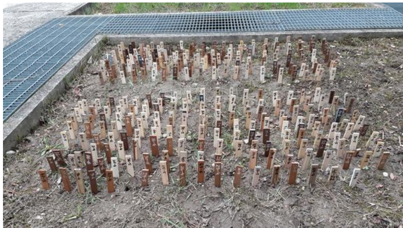
Figure 3: Facades materials during degradation in soil – simulation of landfilling
