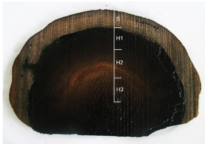
Figure 1: Cross-section of waterlogged archaeological oak wood divided into four zones: S – sapwood, H1 – outer heartwood, H2 – middle heartwood, H3 – inner heartwood
