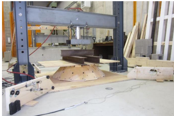
Figure 4: Compressive test of A (lower) level of dome-shell. (Photo T.Teppand).
