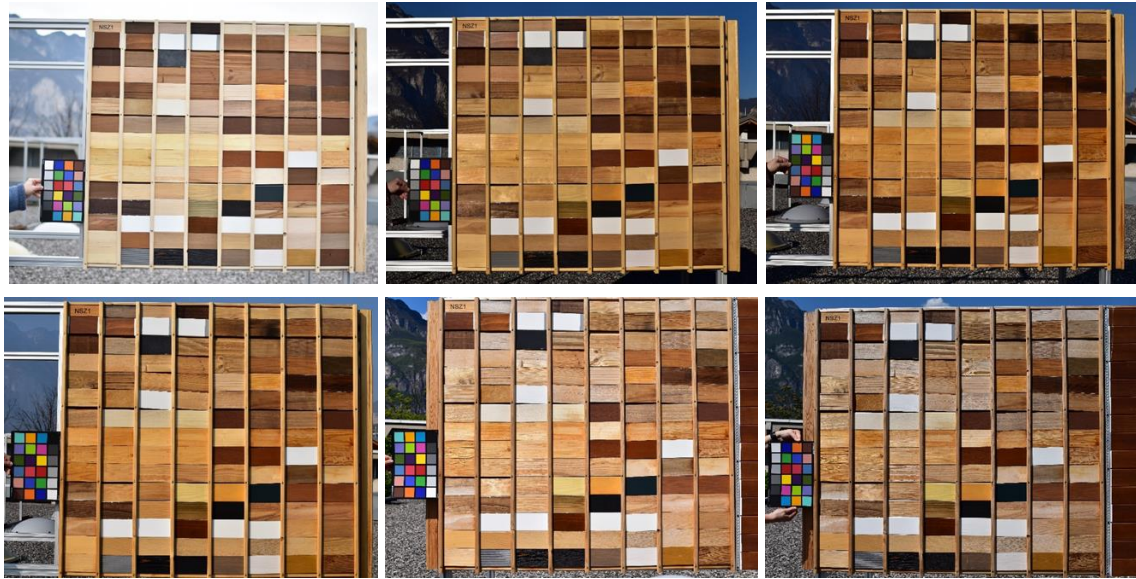
Figure 2: Facades materials at the beginning of weathering test, and their appearance with the progress of weathering (up to 5 months).
