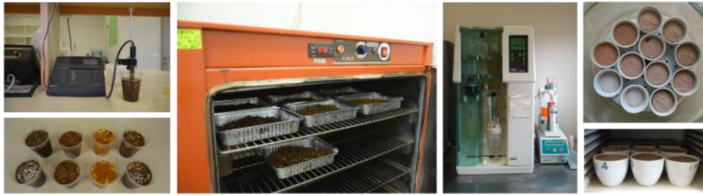
Figure 2: Chemical parameters tests (from left to right); pH and electric conductivity, water, nitrogen and ash contents.
